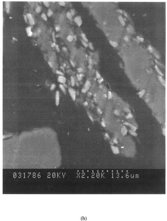
Fig. 1 (a) Cross section of an Al-50SiC8 powder milled for 1800 s with process control agent (PCA) as an additive. (Art has been reduced to 43% of its original size for printing.) (b) Cross section of an Al-50SiC8 powder milled for 1800 s without PCA. (Art has been reduced to 42% of its original size for printing.)
